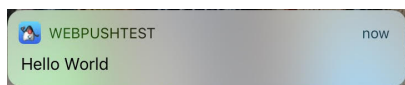
Figure 383. Push type 1 "Hello World" message in iOS when app is in background.
